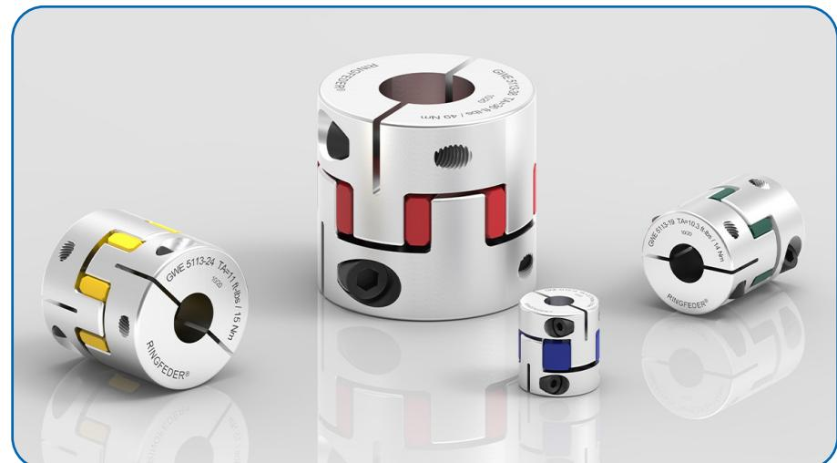
vibration- and shock-damping power transmission, owing to the symmetrical arrangement of the clamping slots and screw positions, as well as the unslotted cam area.
