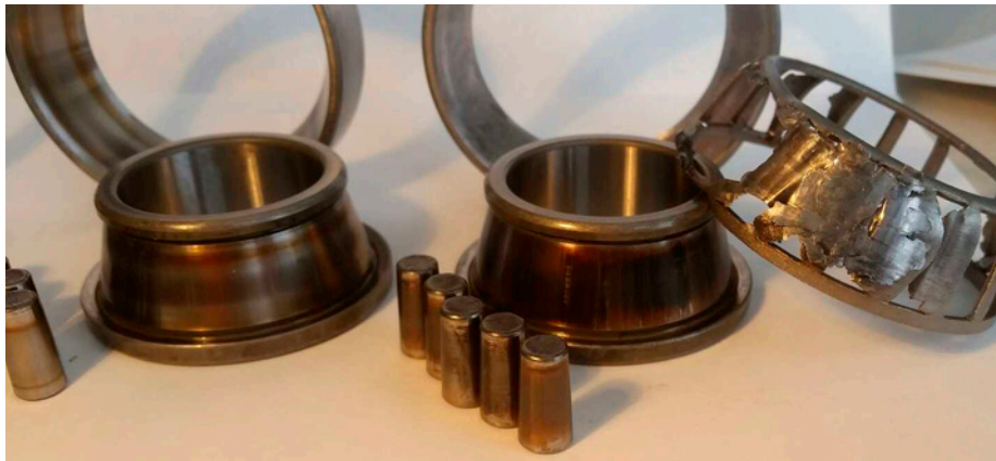
Image 1—Bearing Failure from an improperly grounded test cell.
