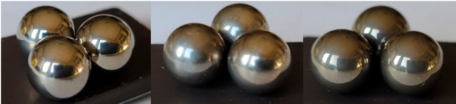
Figure 7—A Range of Ball Conditions: 7a (new), 7b (light dulling), 7c (opalescent).
