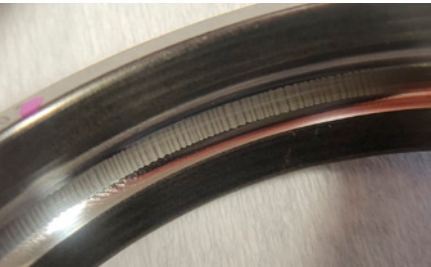
Figure 8—Heavy tactile fluting on motor bearing (picked up on vibration sensor).
