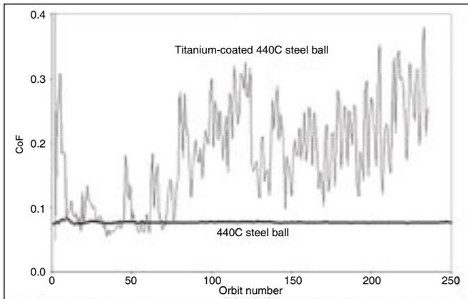
**Figure 10—Friction traces of a system with a 440C steel ball and a 440C steel ball coated with a thin film of titanium. Both balls have been lubricated with ~ 25  $\mu\text{g}$  of Pennzane oil and run on 440C steel plates.**
