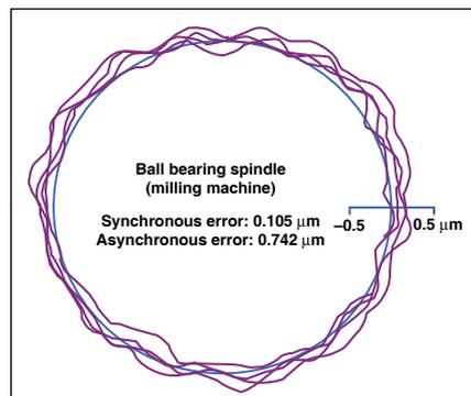
**Figure 6—The ball bearing spindle shown here has more than 100 nm of synchronous error, and the asynchronous error is a large multiple (7X) of the synchronous error. This is why an air bearing spindle (Fig. 5) diamond turning or fly cutting machine can produce a mirror surface finish, while the rolling-element spindle lathe or milling machine cannot.**
