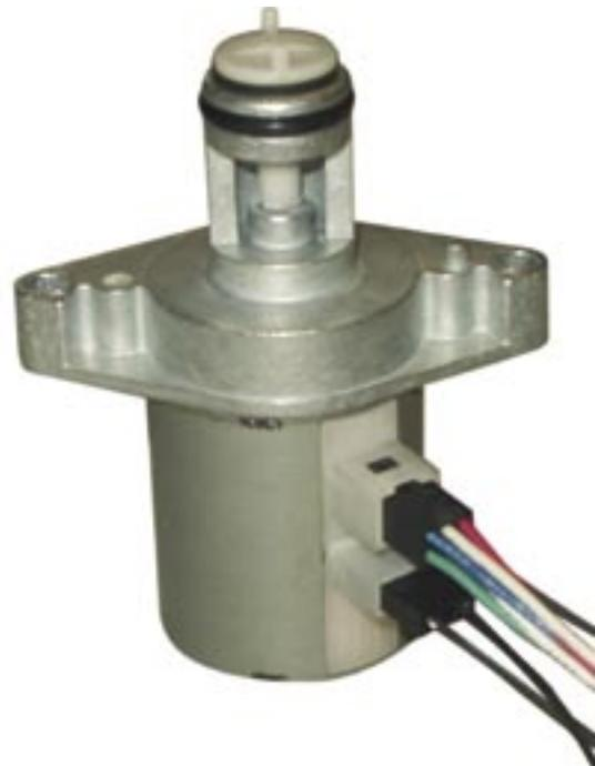
forces are available in the series. They each have a standard linear travel of 10 mm, and versions with an anti-rotation device built in can travel up to 35 mm. The first model in the series features synchronous motor technology and offers low- and high-speed connections. It provides 10 mm displacement at 115 volts, a linear step speed of 0.833 or 1.67 mm per second and output force between 27 and 45 N.
