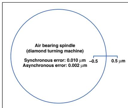
**Figure 5—The difference between fluid film spindles and rolling element spindles is intuitively obvious when compared in error-motion polar plots (see also Figure 6). Notice that the air bearing spindle shown here has synchronous error of only 10 nm, and asynchronous error is a small fraction of that.**
