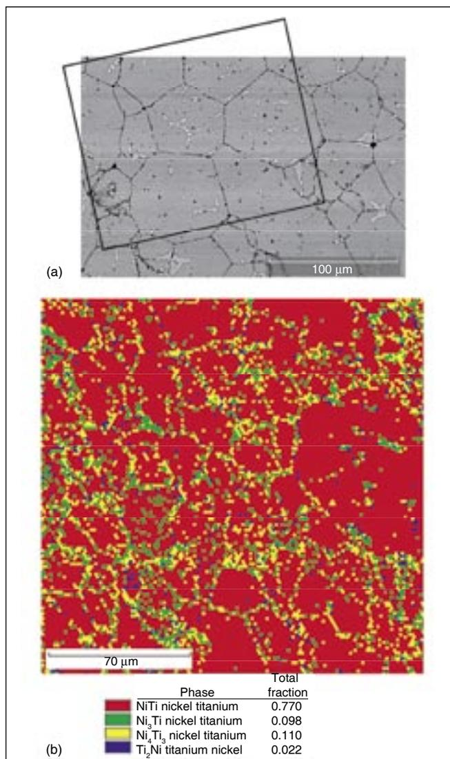
**Figure 3—(a) High magnification micrograph and corresponding area image analysis (outlined box shows analyzed area). (b) Area image analyses of 60NiTi cross section showing discrete phases and their relative proportions based upon area fraction.**
