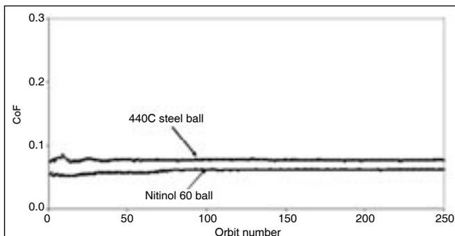
**Figure 12—Initial friction traces of a system with a 440C steel ball and a Nitinol 60 ball. Both balls have been lubricated with ~ 25  $\mu\text{g}$  Pennzane.**
