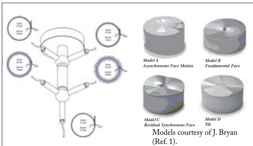
**Figure 4—This illustration shows polar plots generated from the individual signals of each of the five probes shown in Figure 3. The blue band thickness indicates the amount of asynchronous error motion, and the black line shows the synchronous or average error motion. Notice that tilt error motion causes both the synchronous and asynchronous radial error motion plots to double in their amplitude at the outboard spherical target (courtesy of Dr. Eric R. Marsh).**
