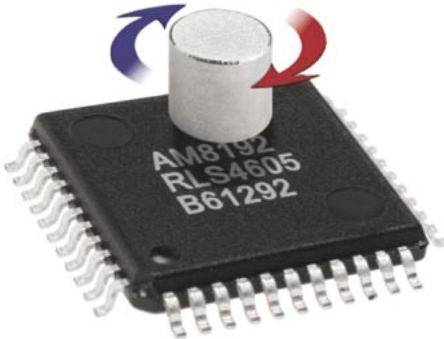
encoder gives OEMs reliable solutions for difficult and extreme operating conditions. Sine and cosine voltage outputs vary with magnet position, which the encoder's interpolator converts to a range of binary and decimal resolutions. It's also able to cancel magnetic interference, permitting operation in areas of high external magnetic fields.
