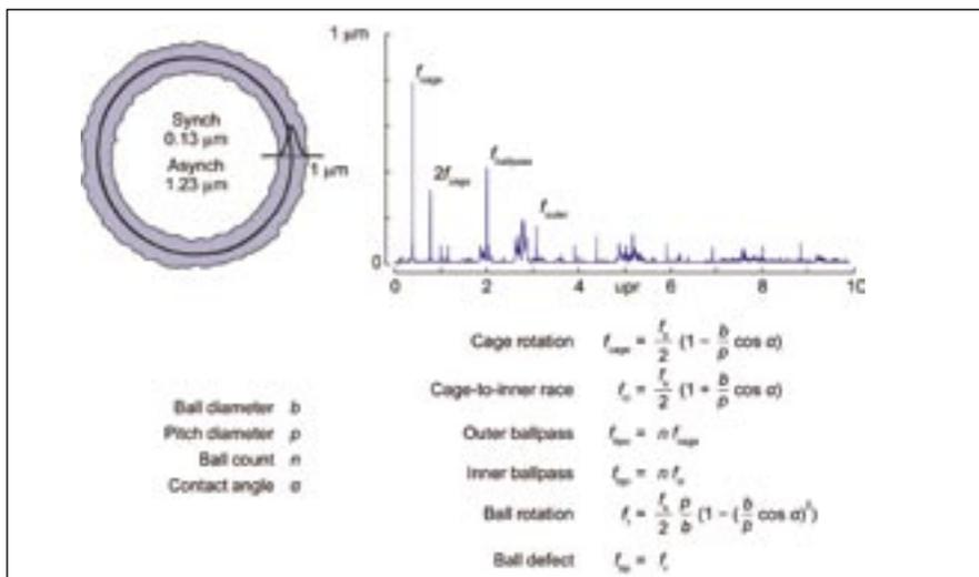
**Figure 8—The above illustrates equations for calculating errors based on the relative size and number of constituent elements. A typical error motion polar plot, top left; and an FFT plot showing frequency spikes of critical elements, top right (courtesy of Dr. Eric R. Marsh).**
