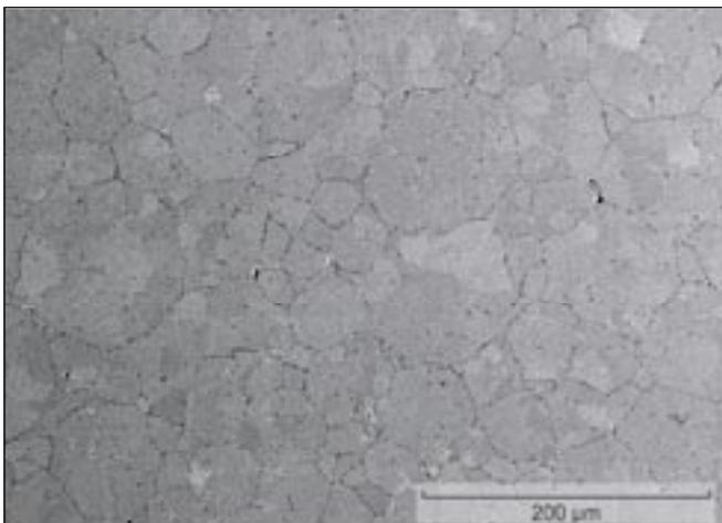
Figure 2—Cross section photomicrograph of 60NiTi ball showing grain structure typical for powder metallurgy processed materials.
