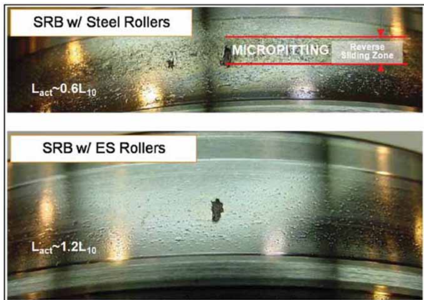
Figure 5—Debris-damaged spherical roller bearings after fatigue life testing in low-lambda. Although micropitting is clearly evident on the ring raceways that ran against uncoated steel rollers, no micropitting occurred on the raceways running against rollers with Timken's engineered surfaces.
