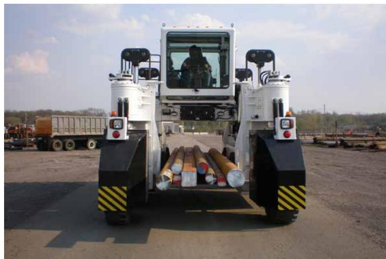
Great Lakes Power's ST35 straddle carrier also utilizes a Mico electrohydraulic braking system.
