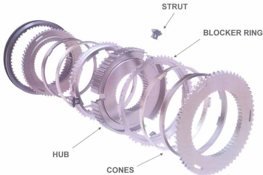
The new synchronizers improve the shift process during three distinct phases:
