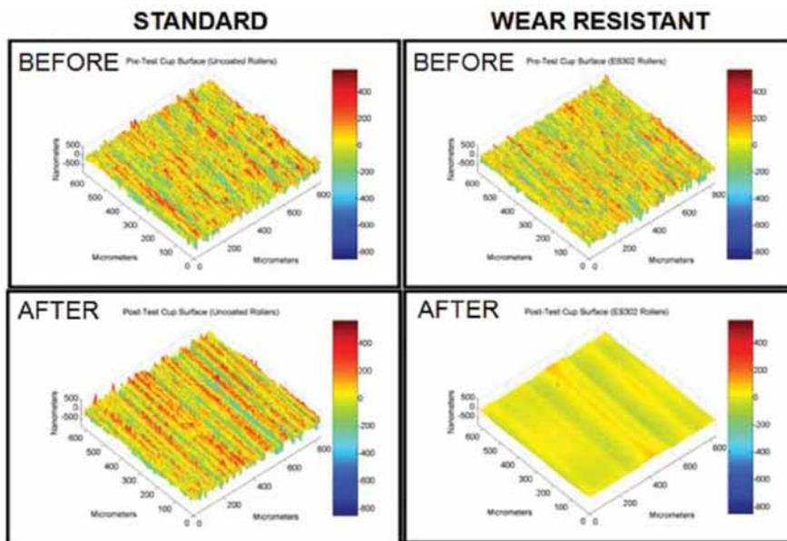
Figure 12—3-D topographical profiles of standard and wear-resistant bearing raceway surfaces before and after completing 44 million revolutions at 150%-rated loads.
