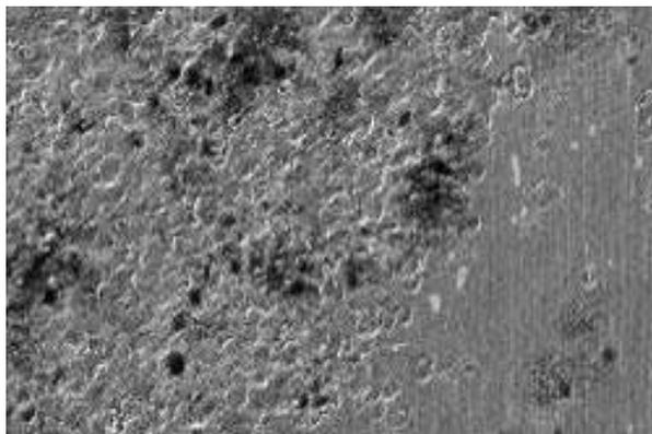
Figure 2—Pitting of a bearing race wall (magnified).
