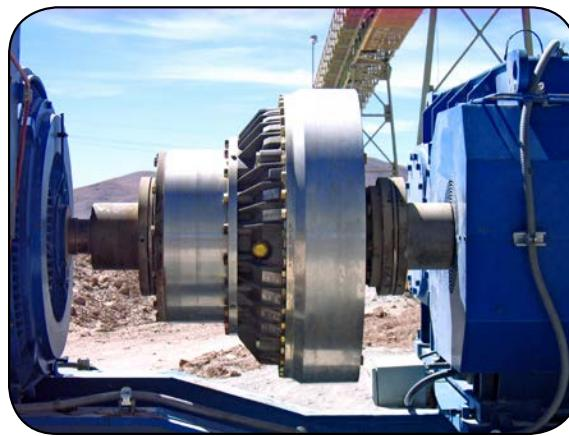
The TVVS constant-filled fluid coupling is particularly suited for medium and long belt conveyors with start-up times up to 45 seconds. Fluid couplings automatically match the demand torque of the driven conveyor. The smooth application of fluid coupling torque provides a smooth belt start-up to protect the belt from damaging stresses, thus reducing system downtimes.
