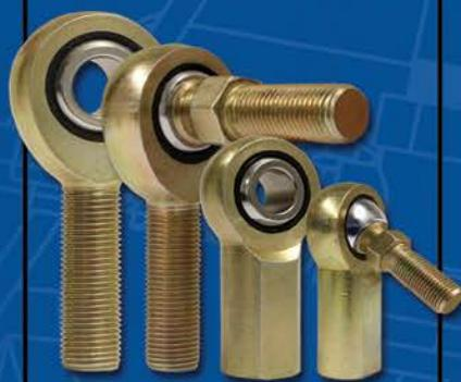
QA1's N Series rod ends feature a molded race compound and low moisture absorption to provide low friction and keep the bearing moving freely. Available in multiple sizes and styles, including male and female, right and left hand threads and with optional studs. These rod ends are self-lubricating, wear resistant and won't bind in damp conditions. Get connected with QA1.
