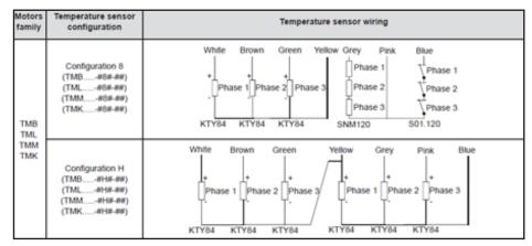
Figure 4 There are two kinds of standard temperature configuration ETEL utilizes for its torque motors.
