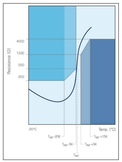
SNM sensors are typically used in low-voltage circuits. Figure 3
