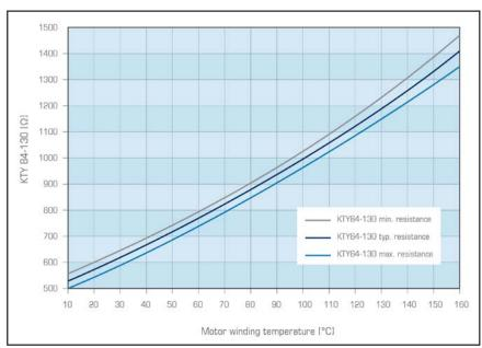
Figure 2 KTY sensors are silicon temperature sensors that have resistance values that change based on its temperature.
