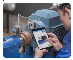
The TKSA 51 consists of two compact and lightweight laser measuring units and shaft brackets to mount the tool, whether on small machines with limited space or on larger equipment using supplied extension chains and magnetic holders.
