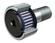
Because the structure of the CFKR series features hexagon holes on both stud ends, it can be tightened from the cam follower head or stud end. Variations are available for roller construction (cage or full complement), shape of the outer ring outside the surface (crowned or cylindrical) and seal structure (shield or sealed type).
