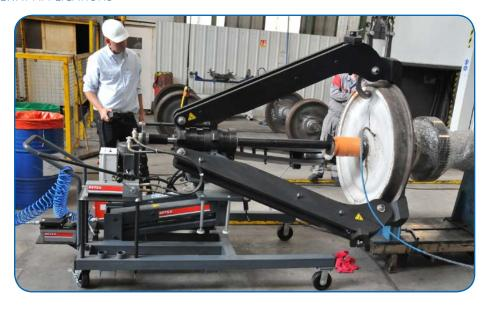
cial induction heaters can be used. Middle frequency induction heating technology is a safe and cost effective heating method that improves the quality of installation. Bega manufactures various models of the Betex MF Quick-Heater, which is also available in combination with fixed or flexible inductors.
