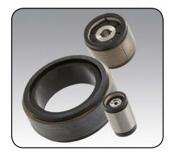
Engineered with ZeroCog slotless motor technology from Applimotion, the effects of cogging torque, magnetic forces, flux harmonics and phase balance and alignment are minimized to counteract the causes of torque ripple. Agility magnetic designs and construction techniques can achieve less than 2 percent torque ripple.
