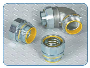
Engineered for applications where sanitation is a critical concern and washdowns are frequent, the UL Listed fittings securely connect flexible metallic electrical conduit while completely sealing off liquids, vapors and solids. A nickel-plated ferrule provides maximum surface contact with longer, more pronounced threads; this ensures pull-out
