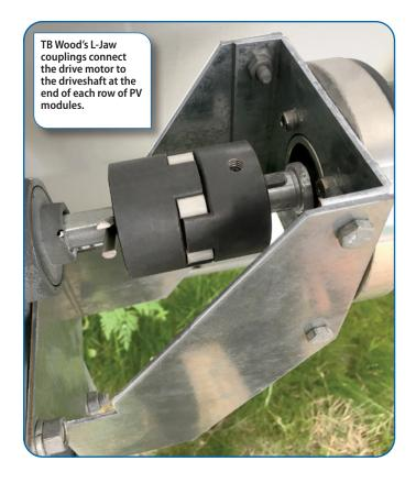
installation and low cost are the primary considerations. These couplings operate with an elastomer element in compression, and they offer a 'fail safe' design (to a degree)," said John Smihal, product manager at TB Wood's. "If the elastomer 'legs' of the 'spider' fail, the coupling can still transmit torque through the hubs."
