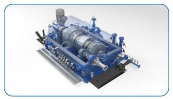
The required specified output speed is achieved by the gear ratio of the parallel shaft gear. Adjustable guide vanes at the pump wheel control the liquid flow in the torque converter and determine the speed of the turbine wheel. This allows the speed of the driven machine to be infinitely adjusted.
