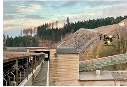
minutes, ConveyorInspect can operate over a maximum range of three miles (5 km) and at a maximum altitude of 400 ft. (130 m). The drone is equipped with a 4K Daylight Camera and 640x512 thermal camera with a frame rate of 30FPS.
