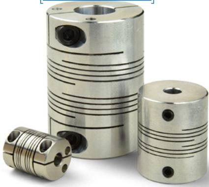
repeatability, and reliability in robotic systems. They have larger body sizes than comparable four-beam couplings for increased torque and torsional stiffness. F-series clamp-style beam couplings are supplied with Ruland's proprietary Nypatch anti-vibration hardware to prevent screws from loosening during operation.
