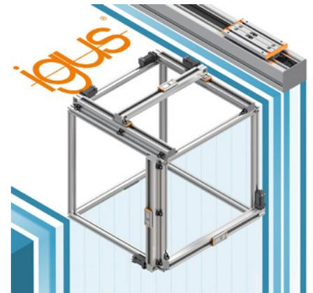
The heart of the new toothed belt axis is the linear guide system from the drylin W series, size 16, integrated into a robust, corrosion-resistant, clear anodized profile. Unlike other igus axes, the toothed belt runs inside the profile, giving the axis the appearance of a mechanical engineering profile.
