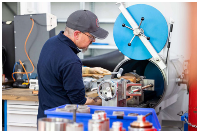
Precision manufacturing of filtration sieves for the Orion spacecraft. (Image: John Crane)
