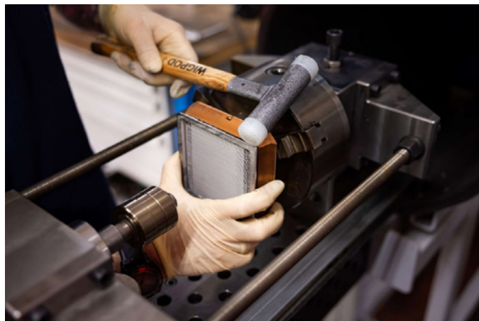
Each filtration sieve is carefully assembled to support reliable propellant management in space. (Image: John Crane)
