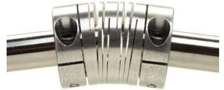
more flexible with lower bearing loads while six beam couplings feature a larger body size with shorter spiral cuts to provide increased torque capability, repeatability, and torsional stiffness. Multiple beam couplings are available in aluminum for additional flexibility and low inertia, or in stainless steel for higher torque and increased corrosion resistance. Special dimensions, spiral cut patterns, finishes, and materials are available by request.
