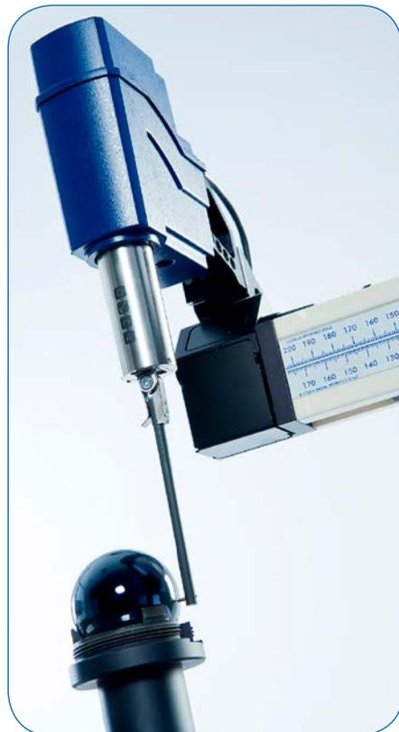
by Taylor Hobson, a unit of Ametek, Inc. The new Talyrond 500H measures roundness, profile and surface finish on a single platform with high accuracy due to an extremely low noise floor. It is ideally suited for high-accuracy measuring applications including precision bearings, fuel injectors, crankshafts and turbocharger parts. Numerous specialized accessories allow the instrument to accommodate the industry's most demanding applications.
