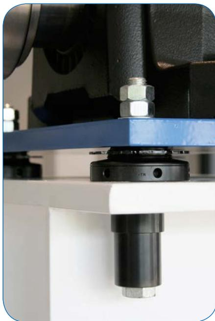
all other heavy-duty bolted joint applications. The all-spherical two-piece washer automatically adjusts under compression to compensate for up to four degrees of angular deviations. This creates an exact parallel plane between the inner face of the bolt head and inner face of the nut to distribute the load evenly over the entire inner contact surface areas. Any need for on-site machining (spot facing) to achieve parallelism is eliminated.
