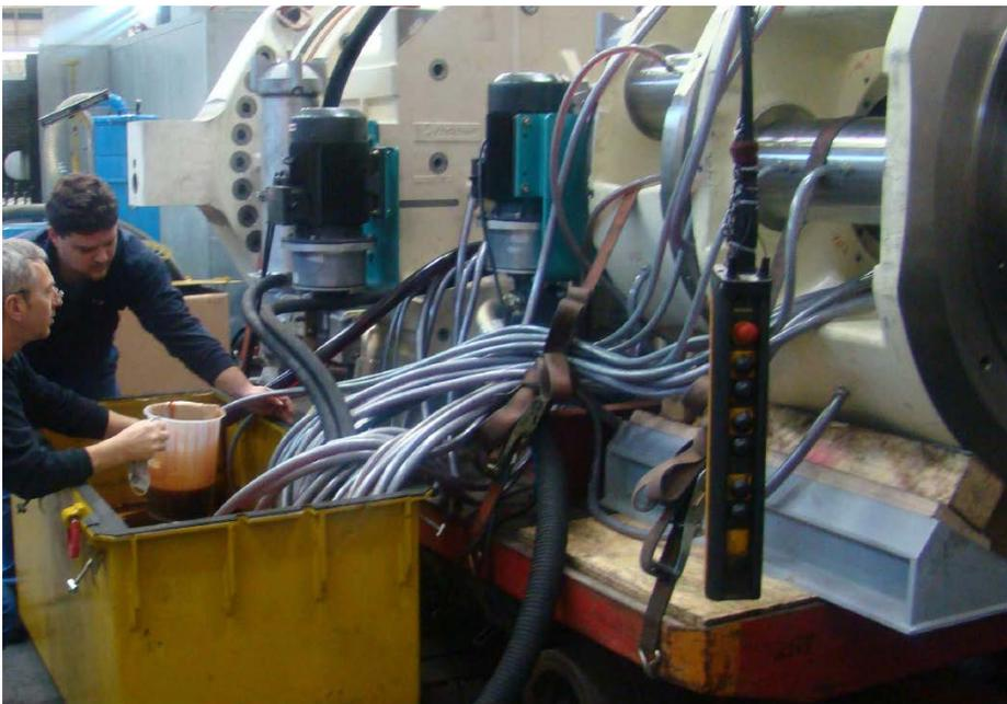
Figure 4 Verification of the specific required oil quantities for toothings and bearings.
