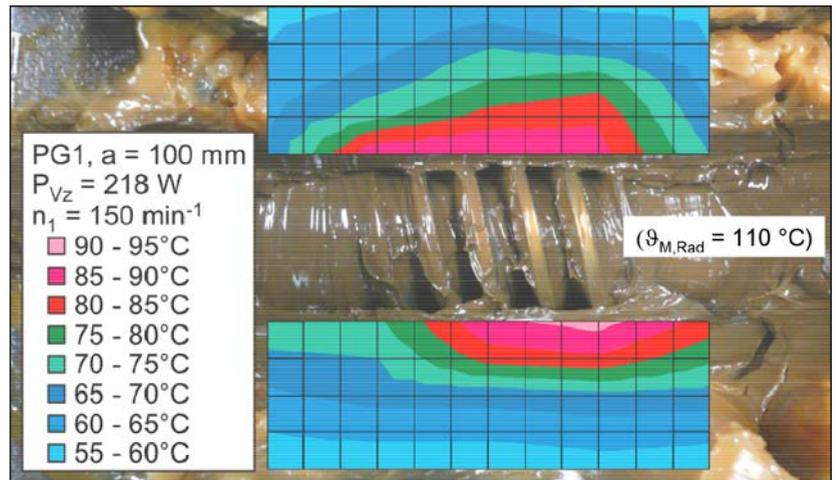
Figure 2 Heat gradient inside gearbox at worm section.
