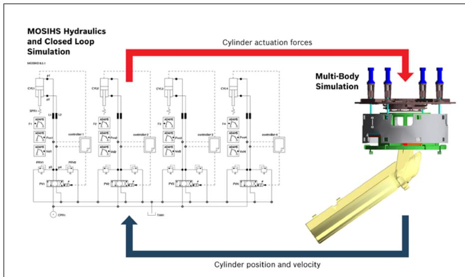
Figure 1 Simulation model of the distributor hydraulic circuit showing closed loop cylinder actuation forces and position and velocity.
