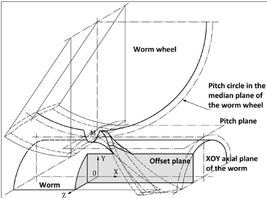
Figure 5 Pitch surfaces and offset plane.
