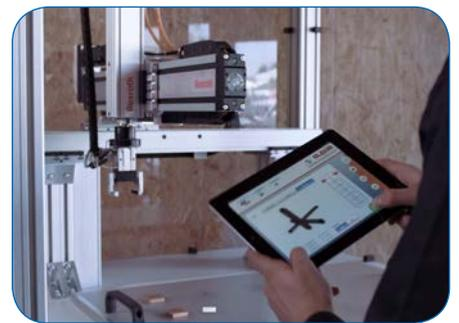
The systems are based on Open Core Engineering with Open Core Interface technology as well as the controls IndraMotion MLC and IndraLogic XLC from Rexroth.
