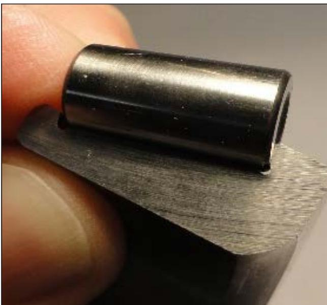
TRB cross-section highlighting rib/roller interface.
