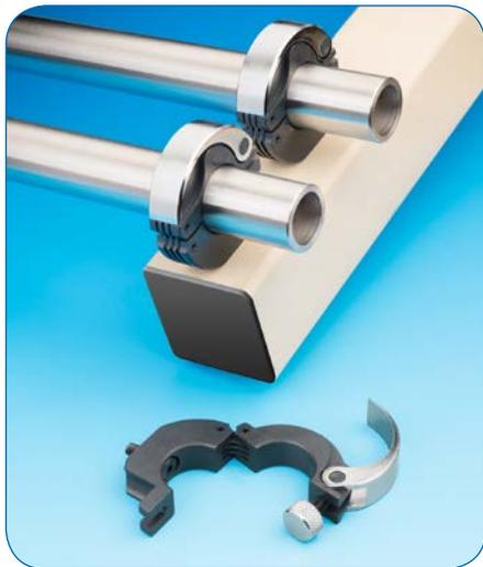
Staff-Lok Hinged Shaft Collars feature an integral hinge with a conformal cam lever for clamping and a knurled nut for adjusting the clamping preset, which makes it easy to open-close and clamp by hand. Now offered with a mounting flat with a countersunk hole and attachment screw, they are ideal for securely mounting pipe and tube requiring frequent or fast changes.
