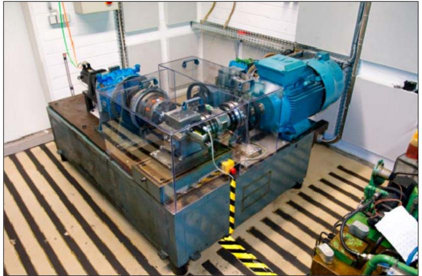
Figure 1 Electrically braced test rig at FZG.
