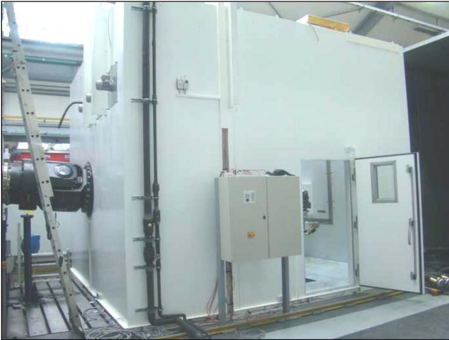
Figure 3 Eickhoff 5MW test rig with climate chamber.
