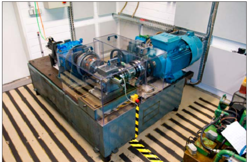
Figure 1 Electrically braced test rig at FZG.
