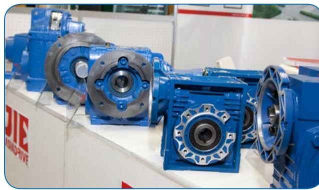
a single- dual-, or triple-stage design. Each gearbox variant is also available as a precision design with reduced backlash. The wide range of sizes and designs allows users to achieve overall transmission ratios from  $i=3:1$  to  $i=512:1$  in a variety of applications.
