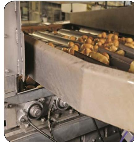
Baldor-Reliance motors and Dodge mechanical power transmission products are designed around food industry sanitation standards with smooth rounded surface textures, minimal crevices and proper sealing for ultimate reliability in environments subject to direct contact with food. Food safe products also undergo stringent testing to carry IP69K for water ingress protection rating for the high pressure, high temperature cleaning methods.
