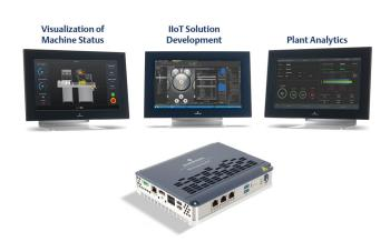
a patented thermal design, enabling 100 percent CPU performance across extreme temperature ranges without throttling. Performance benefits of RXi2-BP are enhanced when paired with PACEdge and Movicon software, providing HMI, historian and analytics applications right at the machine or edge.
