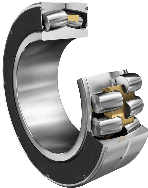
*Sealed spherical roller bearings are designed to keep contaminants out of bearings in manufacturing environments such as mining operations. Schaeffler sealed 241/1250 spherical roller bearings with an outer diameter of 1950 mm operate in one of the world's largest high pressure grinding rolls (HPGRs).*
