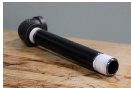
Figure 1—Typical threaded pipe connection with thread sealant.
