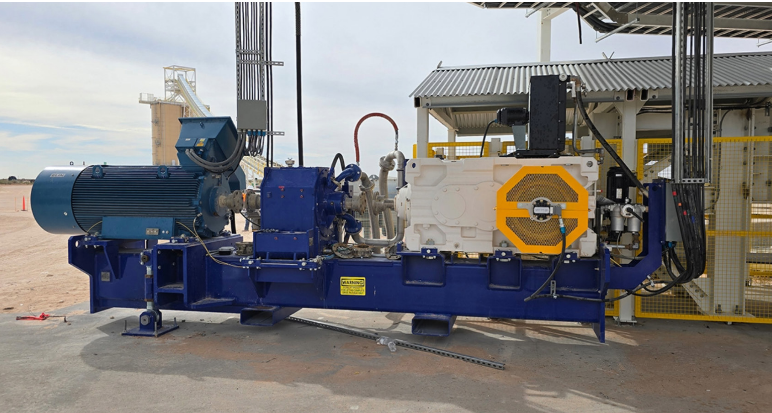
SEW-Eurodrive supplied 36 custom helical-bevel heavy industrial gear units engineered specifically for continuous-duty performance in rugged desert conditions. (Image: SEW-Eurodrive)
