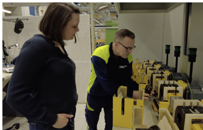
Putting grease to the test: Joakim Hallberg walks Elin Liden through this specific grease life testing setup at SKF Global Testing Sweden.
