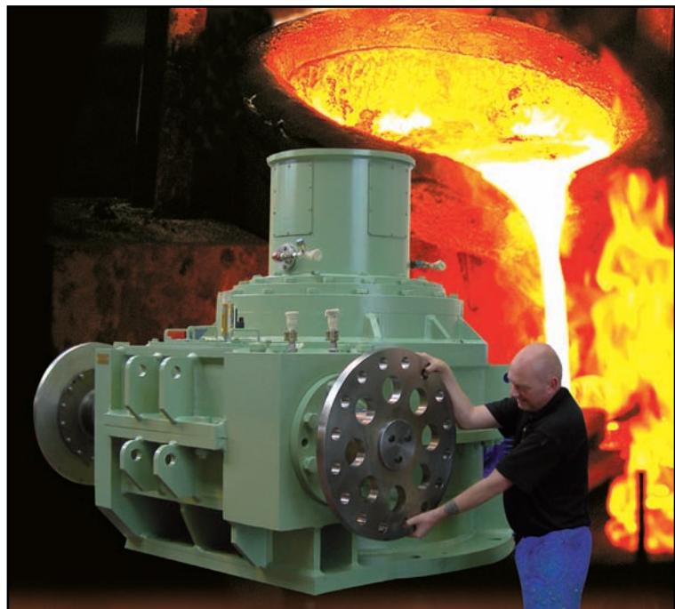
Renold Gears manufactured a pair of wormwheel gearboxes which combined weigh nearly 25 tons. The gearboxes, made for a steel mill in Asia, are the heaviest ever manufactured by the company, according to a press release.
