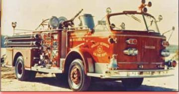
A 1961, 900-Series American-LaFrance 1,000-gpm pumper truck. The engine is by Boeing—a \$10,000 option. The truck was one of three that American-LaFrance built that year and the only one shipped to the East Coast—specifically, to Mount Vernon, Virginia, where Dave Collins worked at the time as a professional firefighter. Note how the clearance between the top of the tire and the front fender opening speaks to how light the engine was. (courtesy Dave Colllins).
