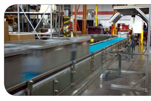
cumulation conveyor with a cleverly designed surface that minimizes load and energy use. We use the accumulation section to spot check our totes for picking accuracy." Automatic sorting to the shipping lanes is planned for late 2012, using scanners and pushers, with manual sortation being used in the short term.
