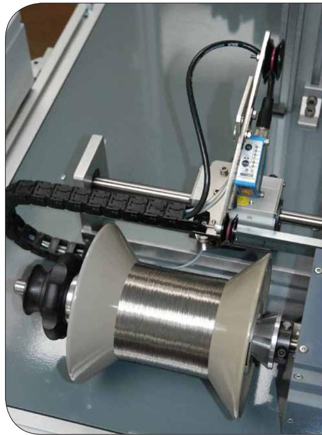
application. Because the distance from the sensor to the sloping surface of the tapered flange is less than the master reference point, reversal is not trig-
