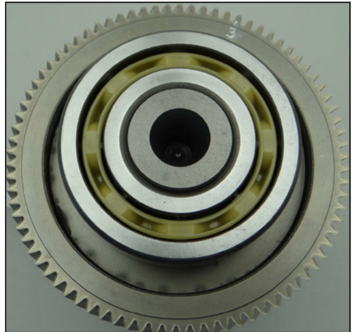
Figure 13 Sinter gear after torsional strength test.
