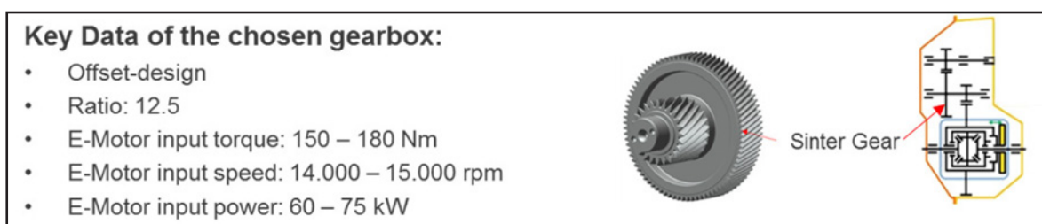
Figure 6 Sinter gear in e-drive gearbox.
