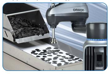
Another key solution for flexible manufacturing is the AnyFeeder flexible feeding system, which will be combined with an integrated controller PLC programmed using Sysmac Studio and running on an EtherCAT as part of a robotic cell demo.
