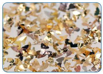
the most advanced materials and manufacturing methods used by the consumer electronics industry to make completely standard, flat, chip-like designs. Then, we just transform them into 3D flying shapes by principles that are similar to those of a pop-up book."
