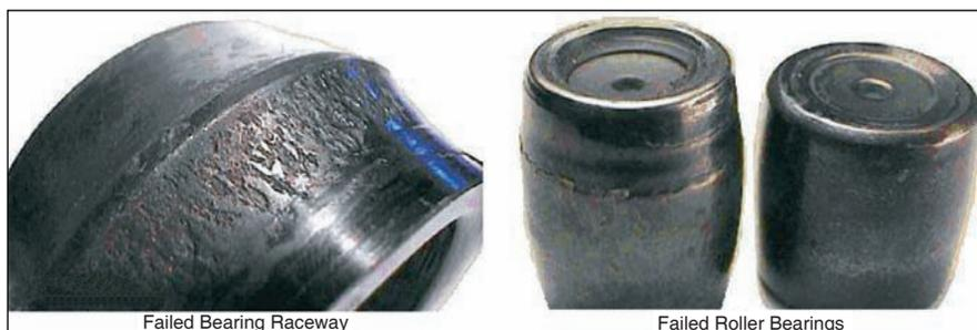
Figure 1—Failed roller bearing elements.
