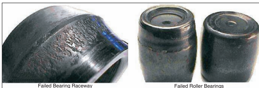
Figure 1—Failed roller bearing elements.
