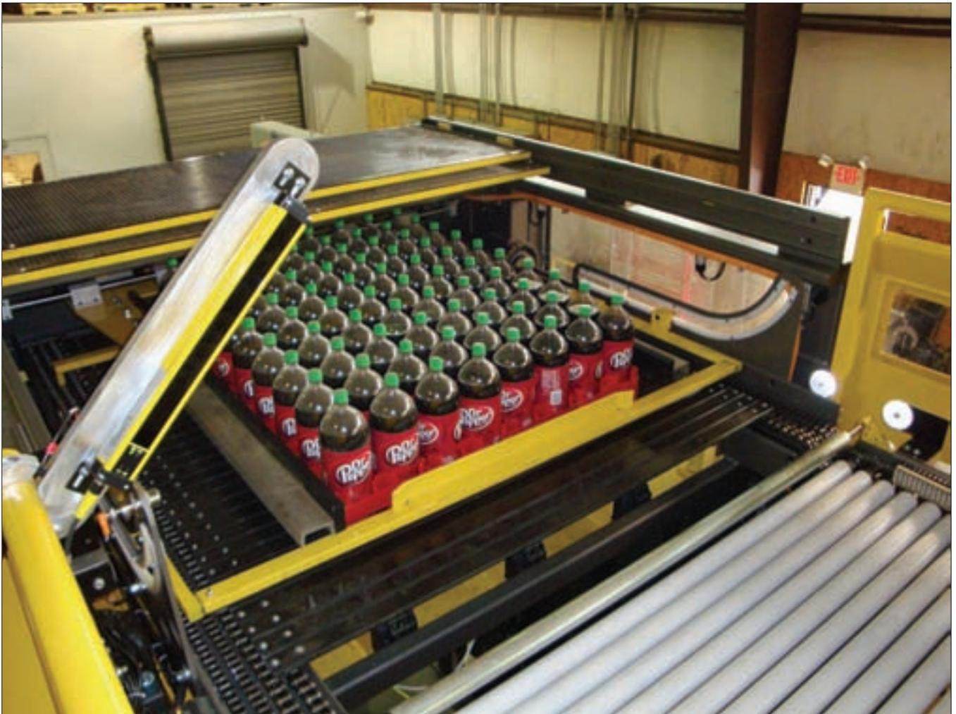
Using Rexroth's IndraDrive M drives and MSK servo motors, T-TEK saw a 15–20 percent improvement in apron and compression cycle times (courtesy of Bosch Rexroth).
