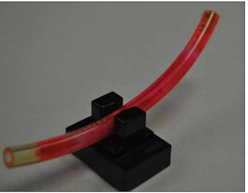
A series of ultrasonic, non-invasive air bubble and particle detectors (above and top, next page) from Cosense has a wide range of applications for the detection of air bubbles and particles in fluid-lines in the wafer etching process as well as in coolant lines. Standard sensors can detect air bubbles as small as 500 microns in size in tubing from 1 mm to 12 mm. Custom sensors for OEM customers can be designed to measure air bubbles down to 100 microns in size (photos courtesy Cosense).
