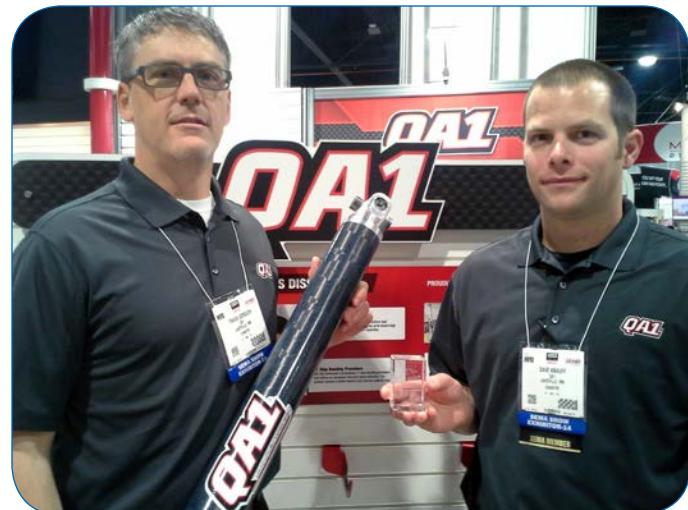
QA1's carbon fiber driveshafts, which are currently offered for street performance vehicles as well as dirt late models, are a major new offering from QA1's Advanced Materials Division. These driveshafts are lighter, stiffer, stronger and safer than aluminum and steel driveshafts and are filament wound in-house using 3MTM Matrix Resin that is exclusive to QA1 performance driveshafts.
