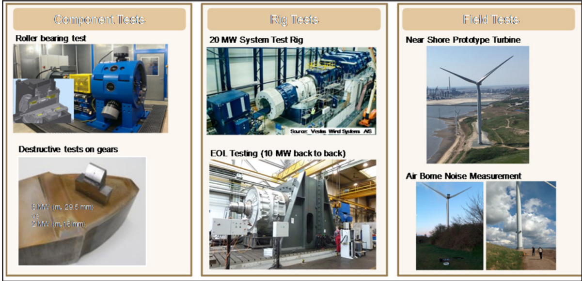
Figure 8 Validation procedure with component, system and field tests.
