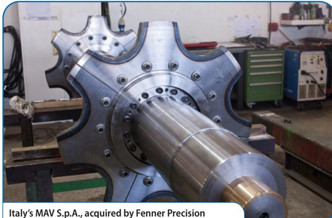
Italy's MAV S.p.A., acquired by Fenner Precision Polymers on December 1, 2020, produces a wide variety of engineered solutions like the keyless locking device shown here, used in apron feeder applications.
