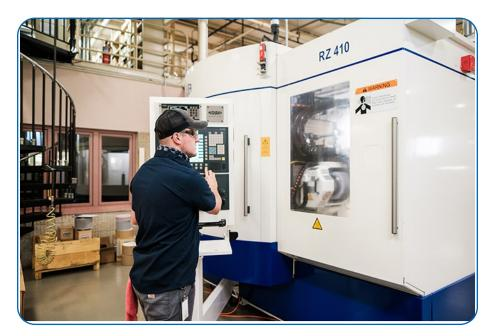
also gives Forest City Gear the ability to perform profile grinding using either CBN plated or dressable grinding wheels that can be modified on the machine with an on-board CNC dressing unit, working in conjunction with integrated inspection.
