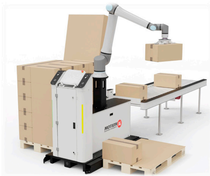
Figure 3—End of line palletizing is the perfect example of a labor-intensive job that can be done with cobots. Image courtesy of Motion Automation Intelligence.
