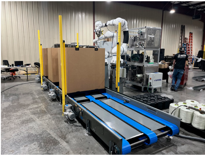
A robot spots a product on a moving conveyor, determines its exact position, picks it up and places it into a waiting assembly, carrier tray or shipping container.
