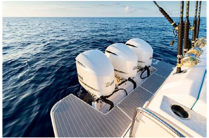
Typical outboard aft platform
