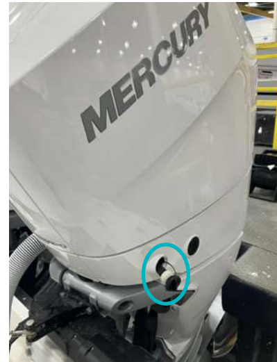
Mercury flush location
