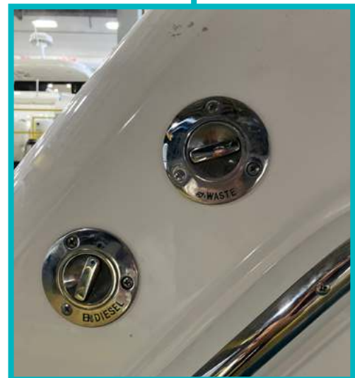
Diesel fill fitting and waste pump-out
