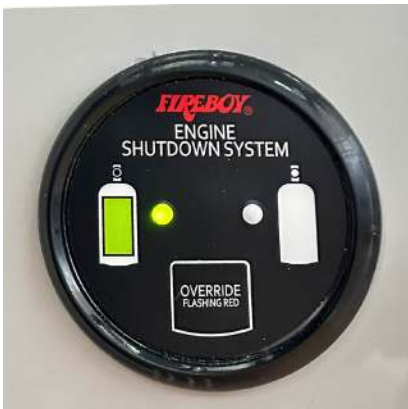
Fireboy shutdown panel
