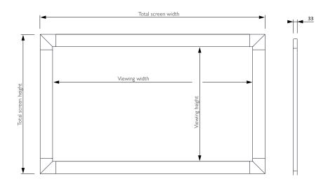
Total frame width = Viewing width + 200mm
