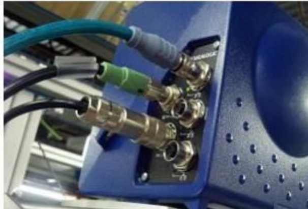
Figure 41: Connections to the DM3610 Connector Panel
