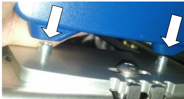
Figure 74: Placing DM3610 on the hollow Spirol™ spring dowel
