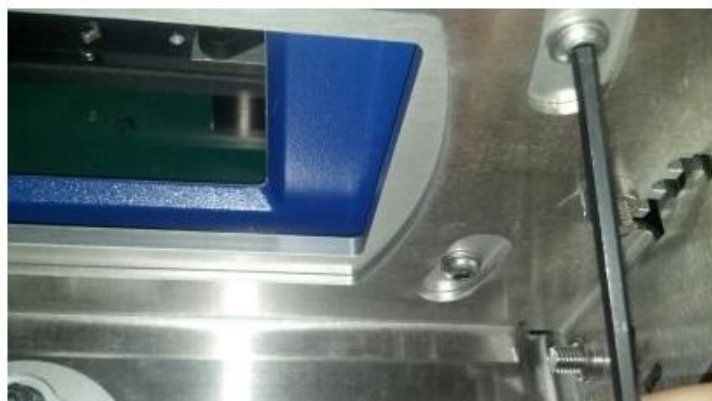
Figure 5.9: Mounting bolt location
