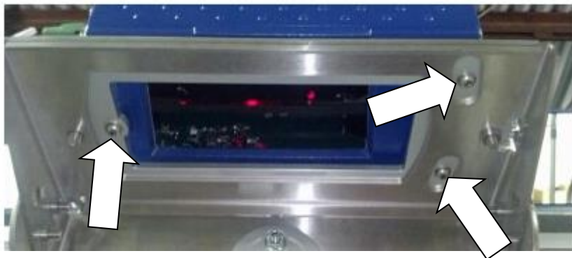
Figure 5.9: Mounting bolt location
