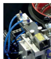
Escapement sensors Control/Secure escapement mechanism
