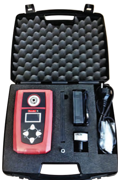
■ Embedded Transducer & Battery
