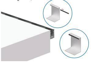
Step 2. Place the aluminum channel to position, and install it with anchor bolts.
