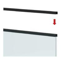
Step 11. (Handrail) Install the end cap of handrail.
