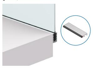
Step 9. (Handrail) Install handrail rubbers on top of the glass.
