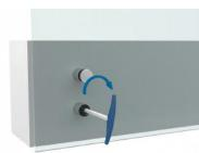
Once the glass is aligned, reinstall the gasket and cover. And use the tool to tighten it.
