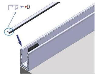
Step 3. Use connector pins between two lengths of aluminium channels, or connect the channel to a 90 degree corner.
