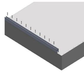
Step 5. Click on the front-side top bead (with rubber gasket)
