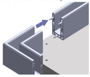
Step 6. Place glass channel into the channel and adjust the alignment between glass pannels
