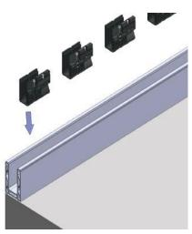
Step 2. Place the aluminium channel to position, and install it with anchor bolts.
