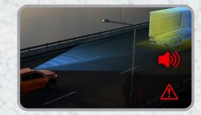
**AUTONOMOUS EMERGENCY BRAKING [AEB]:** Your ISUZU D-MAX ARCTIC TRUCKS AT35 features automatic emergency braking, activated on detection of a potential frontal collision.
