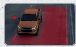
LANE KEEP ASSIST (LKA): Should your ISUZU D-MAX ARCTIC TRUCKS AT35 start to move out of its lane, Lane Keep Assist (LKA), Emergency Lane Keeping (ELK) and Lane Departure Prevention (LDP) help to correct this and prevent collisions.
