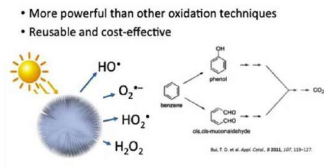
Figure 1. Reaction interface of the catalyst and organic molecules during photo degradation process.
