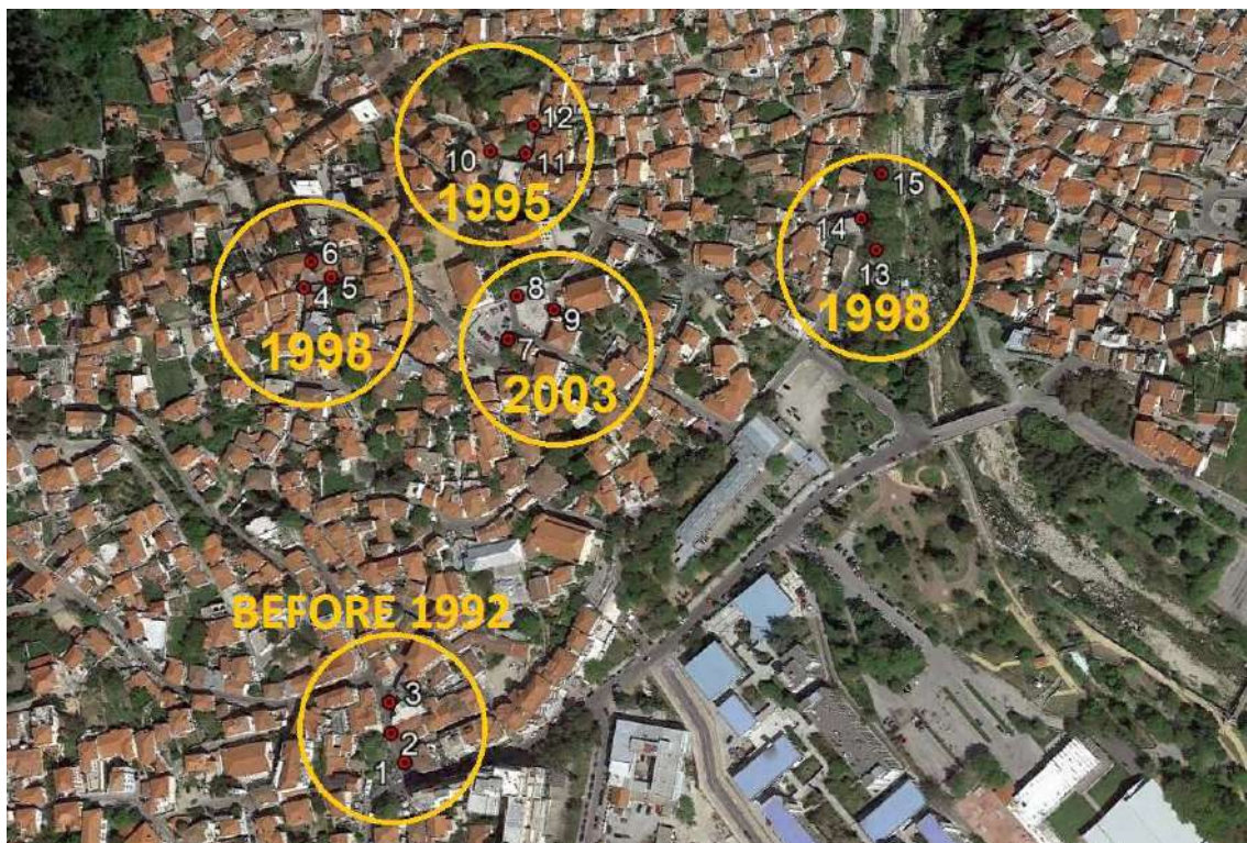
Figure 1. Measurement points and years of cobblestone reconstruction.
