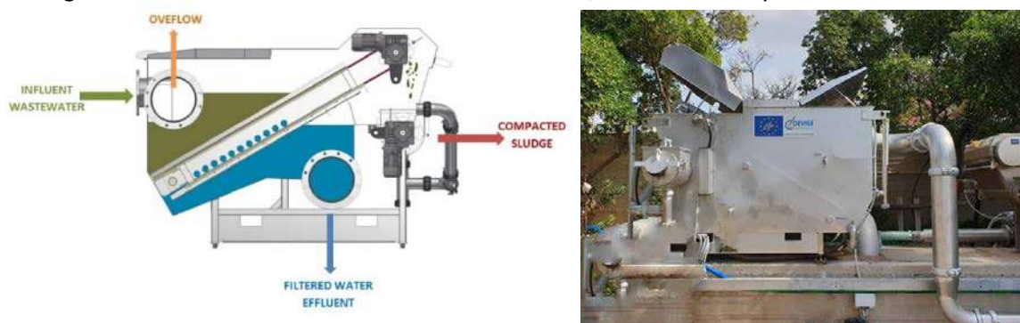
Figure 1. Inlets-outlets of microsieving process (left); Microsieve installed at Rethymno WWTP (right).
