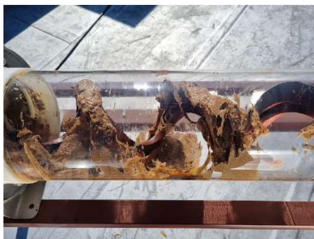
Figure 3. Photograph displaying how synthetic sludge tended to stick to the auger surface.
