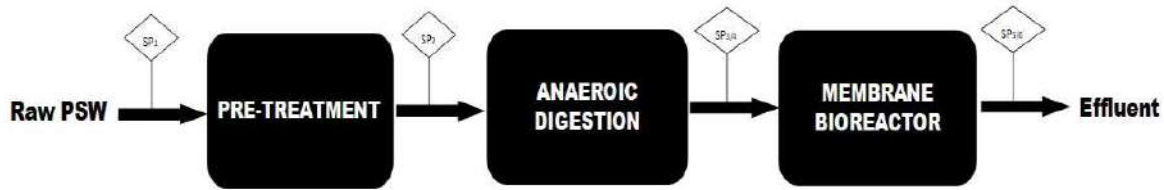
Figure 1: Multi integrated system treating poultry slaughterhouse wastewater.
