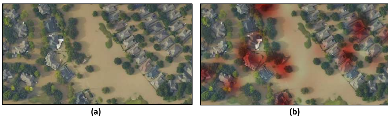
Figure 2. Predictions of our model of a large satellite image: (a) original image; (b) the image with a red overlay showing areas exhibiting increased damage
